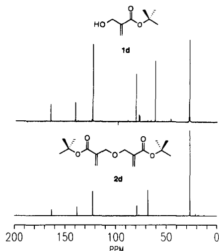
Figure 1. ^{13}\text{C} solution NMR spectra of TBHMA 1d (lower trace) and its dimer ether 2d (upper trace) obtained in \text{CDCl}_3 .
